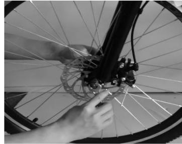
Remove the nuts from the front axle. Slide the wheel into the slots at the end of the forks. If your E-bike is equipped with a disc brake, make sure the disc for the brake slides into the front brake caliber cleanly. Replace nuts and check that the wheel is centered into the fork and the disc is free in the brake caliber. Insure the wheel turns freely. Tighten the nuts with a spanner. **Do not over tighten.**
