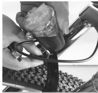
a: Take the screw from the fork, b: Open the lamp c: Install the lamp and tighten.
