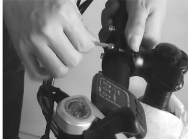
Use inner hexagon tool loosen the stem cover and do not tighten all bolts immediately before adjusting the handlebar in a property angel and position, then tighten.
